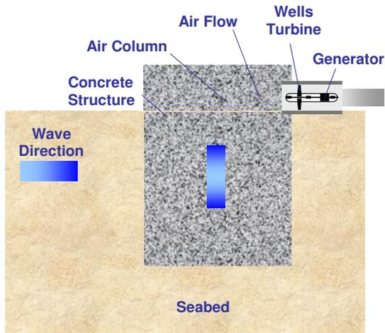
Figure 6: Oscillating water column type of wave device.
