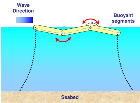
Figure 9: Pitching type of wave device
