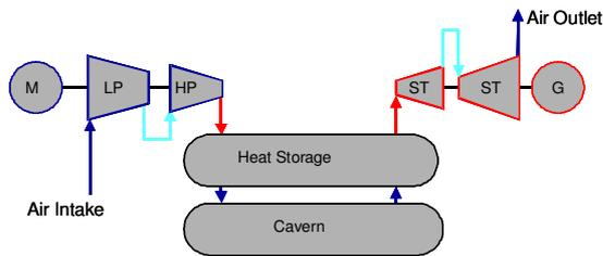
**Figure 4: Adiabatic compressed air energy storage system**
