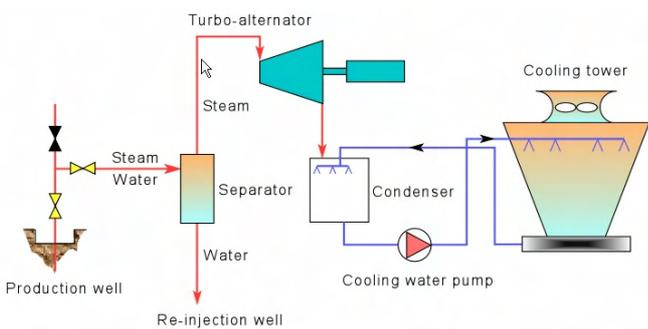
**Figure 7. A schematic diagram of a geothermal condensing power plant**
