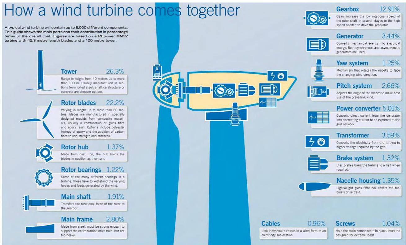
**Figure 6. Example of the main components of a wind turbine and their share to the overall cost in the 5 MW RE Power machine**
