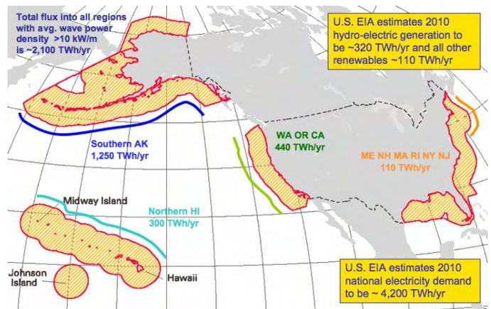
**Figure 2: The wave energy potential expressed in potential electricity production (TWh) at the coasts of US.**
