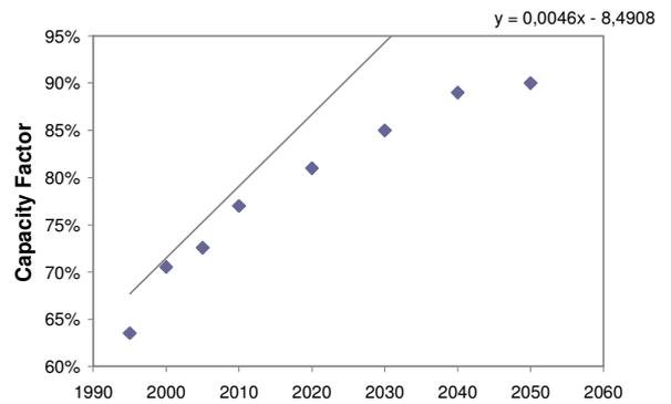
**Figure 20. Capacity Factor of geothermal power plants in the world 1995-2005 and forecasts for 2010-2050**
