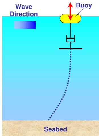
Figure 7: Buoy type of wave device.
