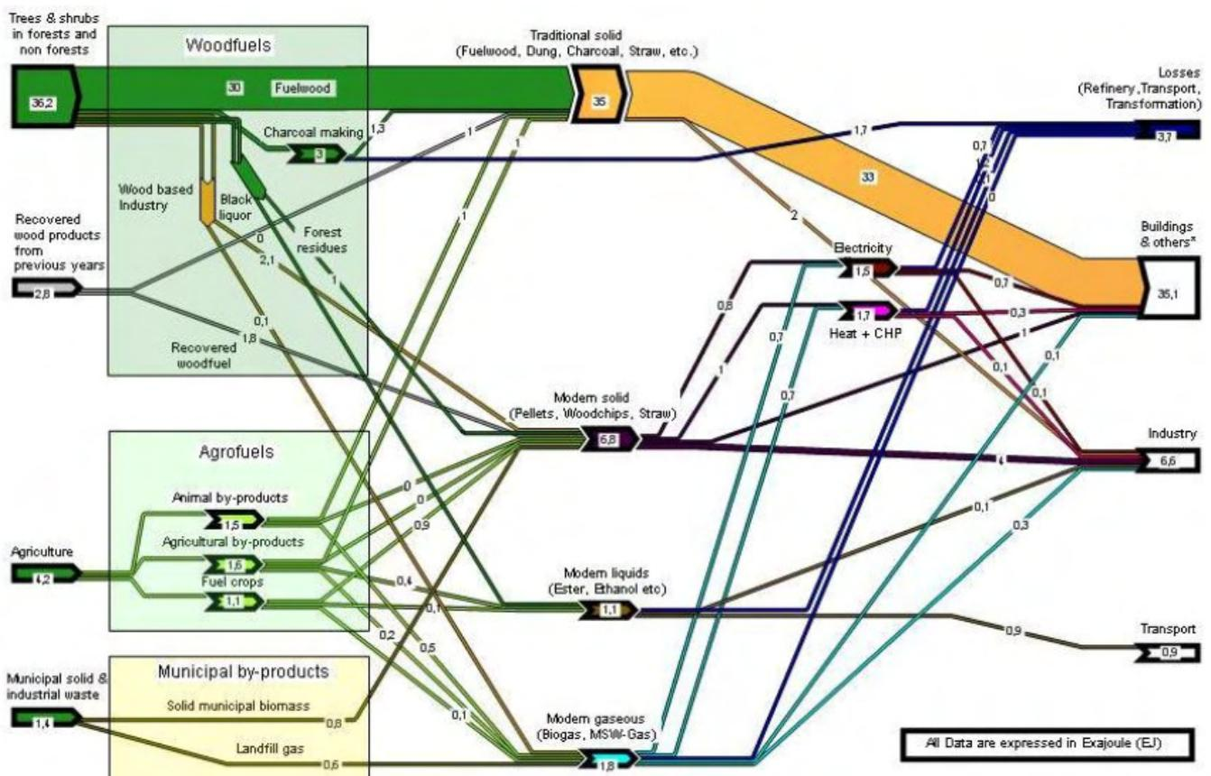
**Figure 1: World biomass energy flows (EJ/yr) in 2004 and their thermochemical and biochemical conversion routes to produce heat, electricity, and biofuels for use by the major sectors.**
