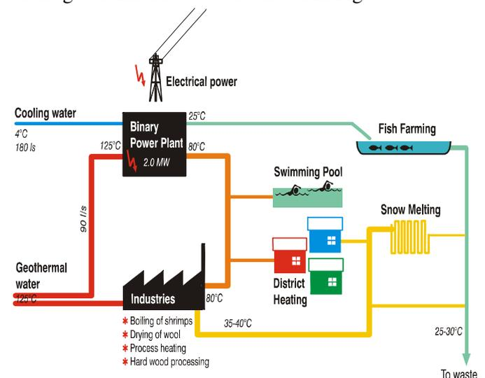
**Figure 8. An idealized diagram showing cascaded uses of geothermal energy.**
