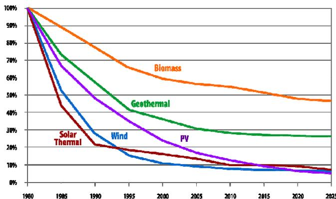
**Figure 8. Past improvements in R&D on various renewable technologies, including solar thermal (red curve) and photovoltaics (purple curve), have yielded impressive cost reductions.**
