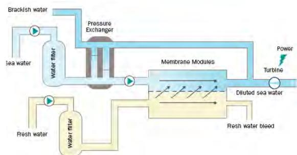
**Figure 11: Diagram of pressure retarded osmosis (PRO) process using salinity gradients.**
