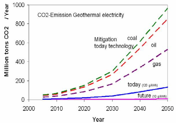
**Figure 21. Mitigation potential of geothermal power plants in the world based on data of Table 6 and assumptions for emission of 120 g CO<sub>2</sub>/ kWh for today and 10 g CO<sub>2</sub>/ kWh for future technology.**
