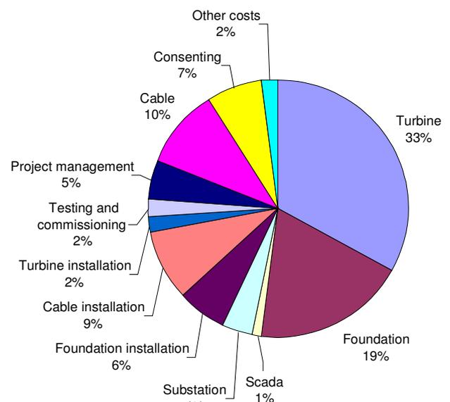
**Figure 9. Estimate of capital cost breakdown for an offshore wind farm**
