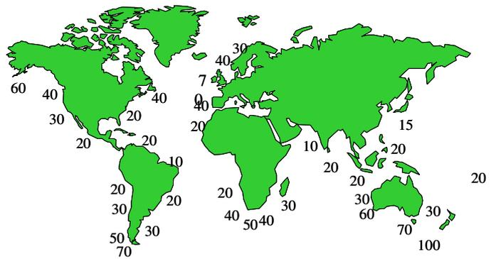
**Figure 1: The highest wave activity (kW/m) is found between the latitudes of ~30° and ~60° on both hemispheres.**
