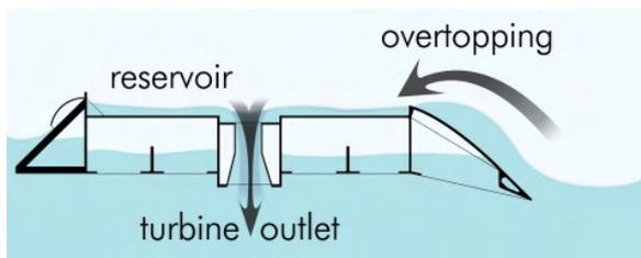
Figure 8: Overtopping type of wave device
