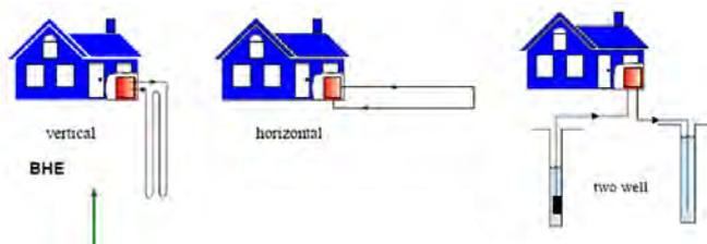
**Figure 11. Closed loop and open loop heat pump systems.** The green arrow indicates the most common system, with borehole heat exchangers (BHE). The heat pump is shown in red. (Modified from Geo-Heat Center, 2008).
