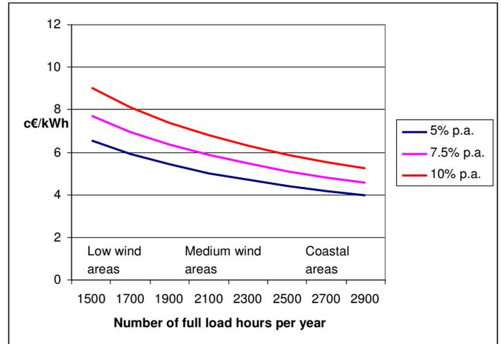
**Figure 8. The costs of wind-produced power as a function of wind speed (number of full load hours) and discount rate.**
