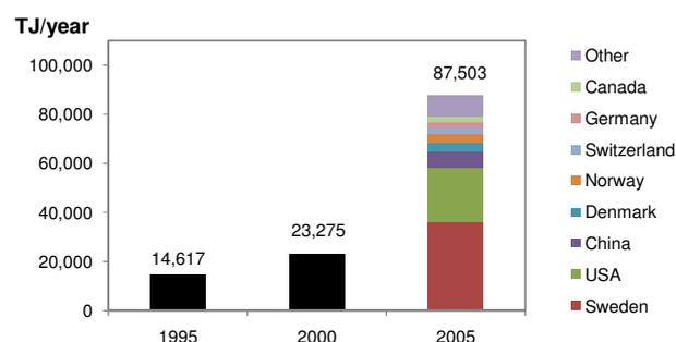
**Figure 13. Worldwide growth of ground source heat pump applications and the leading GHP countries. Data from Lund et al. (2005).**
