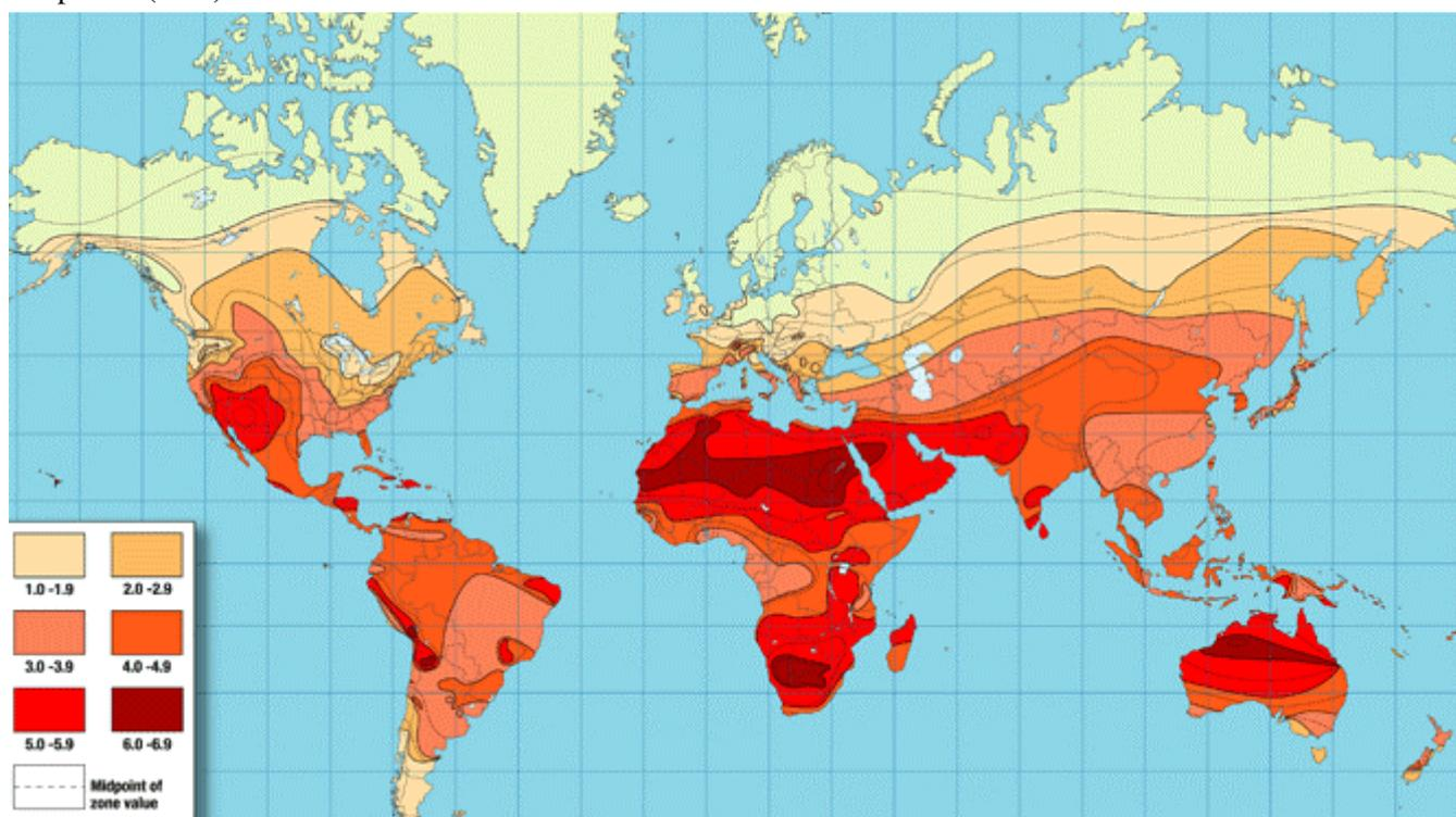
**Figure 1.** The solar resource—sunlight—is robust across much of the world. This map shows the number of hours of solar energy received each day on an optimally tilted surface during the worst solar month of the year [www.howto.altenergystore.com]. The most intense areas of color indicate the most hours of sun.
