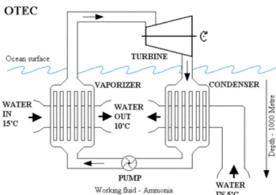
**Figure 10: Diagram of a closed cycle Ocean Thermal Energy Conversion plant**
